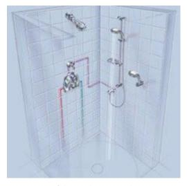
A 3-way transfer valve allows you to use any one of three shower outlets
