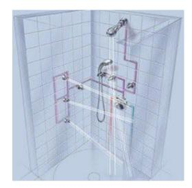
**Two Wall Shower with a Diverter** – The diverter is used to "switch" the from one shower outlet to another. Diverters are less expense than volume controls and are used when:
